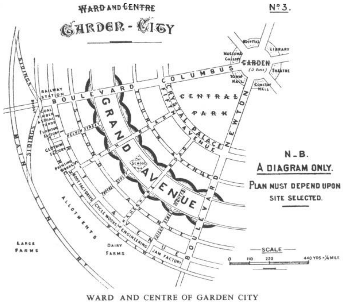
Figure 1.2 - Concentric plan of a typical Garden City, depicting spatial and social hierarchy.
